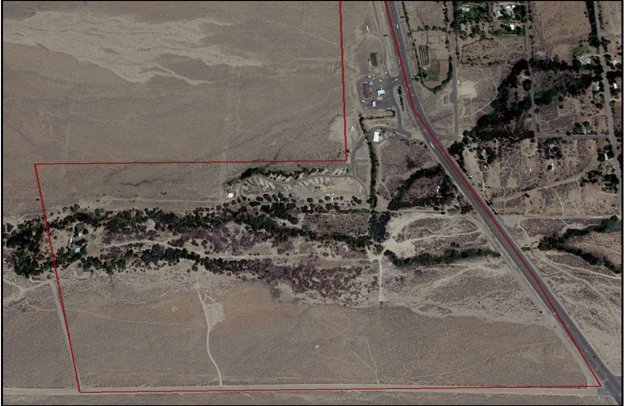
Figure D.7. There are limited roadways in and out of the community, and all are relatively narrow. Roadways are surrounded by flammable vegetation, and there is dense fuel loading along the creek. The red boundary is the community boundary.
