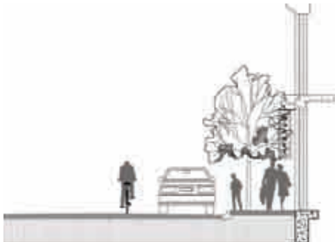
Eight foot sidewalks allow minimal 2-way pedestrian traffic and street furnishings.
