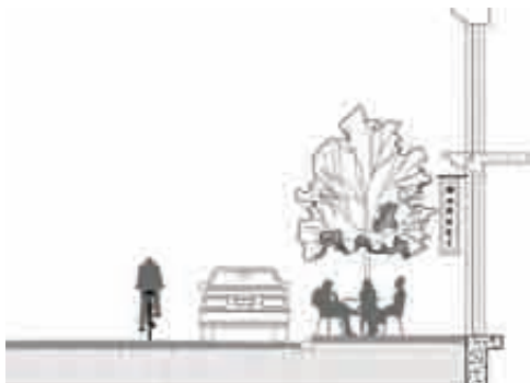
Twelve foot sidewalks allow room for outdoor dining and sidewalk displays.
