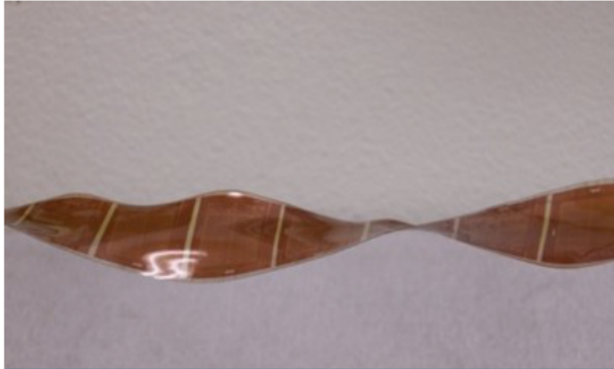
Examples of film distortion caused by advanced Vinegar Syndrome (VS).
