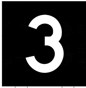
Runway Distance Remaining Sign
