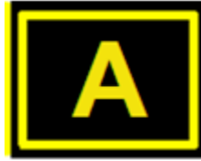
Taxiway Location Sign
