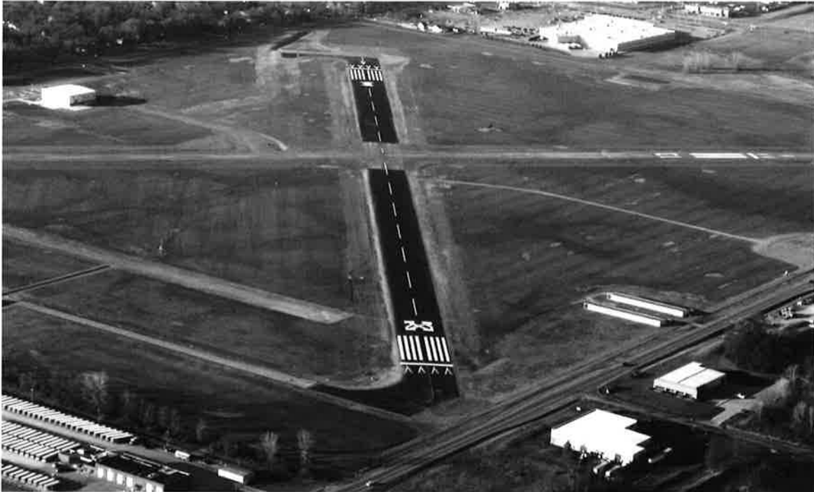
Figure 2-3. Markings for a Temporarily Closed Runway
